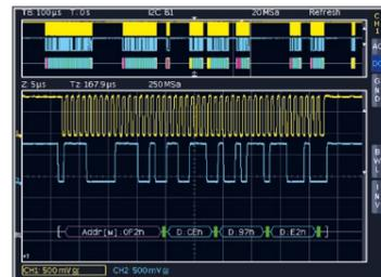
I<sup>2</sup>C bus hex decoding on the analog channel
