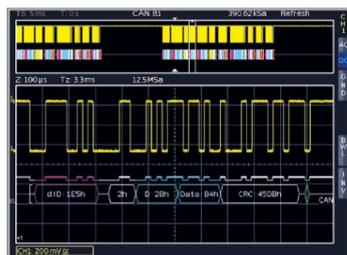
HEX decoded CAN bus signal
