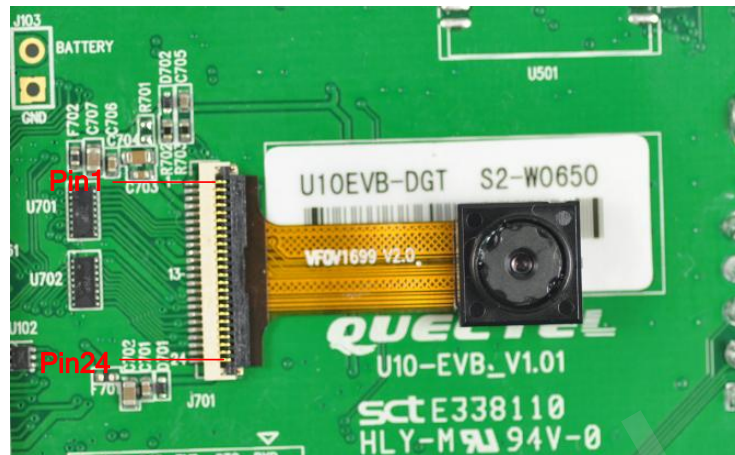
Figure 37: Installation of the camera module.
