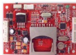
ITM-DVR8100 The DVR81xx is a series of different types of digital video recorders. All types have certain features for certain fields of application. Base module is "DVR8100". Main features are: • Comfortable surveillance functions like motion detection • Applicable for a huge variety of cameras • Taking pictures or recording video • Simple control by display menu • Input and output triggers allow to connect your external applications • Very flexible by custom made extensions (like key board)
