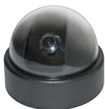
CCTV DOME Camera CCD(Sharp) Color Dome Camera, 1/4" CCD Sensor, 420 TV Lines, 1.0 Lux/F2.0, S/N Ratio >48db, very simple installation with BNC connections
